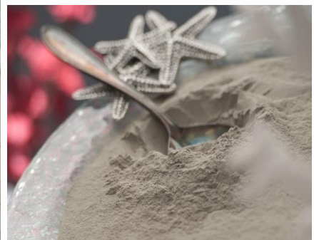
Organic material, sand and larger particles are all screened out to produce an Ultra-fine Clay
