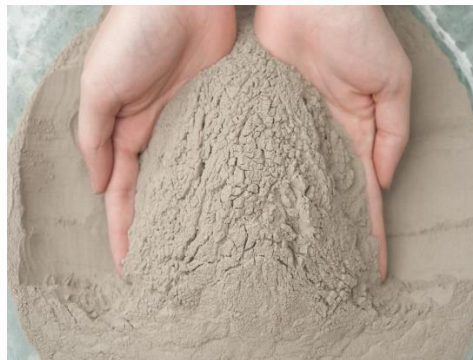
Organic material, sand and larger particles are all screened out to produce an Ultra-fine Clay
