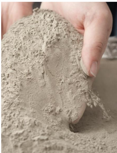
Organic material, sand and larger particles are all screened out to produce an Ultra-fine Clay
