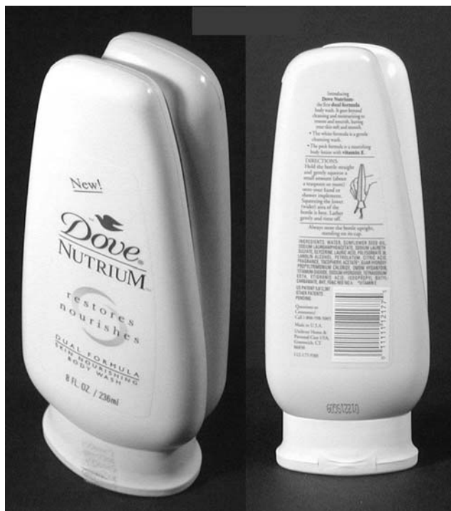
FIGURE 2 Dual dispensing package utilizing two separate bottles attached to each other and dispensed through a single large oval flip-top cap with two orifices. (Courtesy of Unilever Corporation.)
